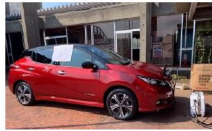
Power supply from EV: Using the EV for mobile phone charging, electric fans, refrigerators, etc. at evacuation shelters, etc. Source: Nissan Motor Corporation
