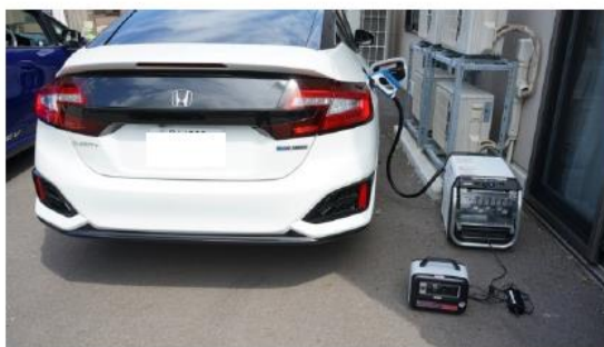
Power supply from FCV: Using the FCV for charging air conditioners and small storage batteries in old people's homes Source: Honda Motor Co., Ltd.
