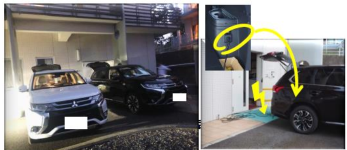
Power supply from PHV: Using the PHV for washing machines and washer / dryers in old people's homes Source: Mitsubishi Motors Corporation
